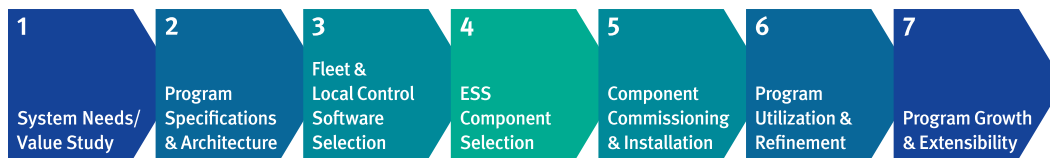
Figure 8. The seven key steps for taking a program approach to energy storage.
